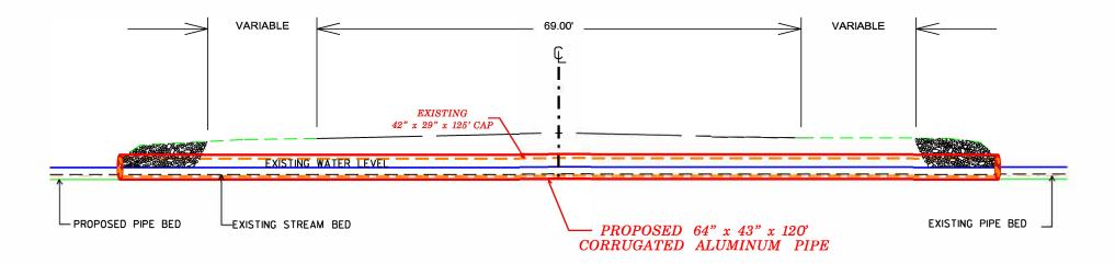
NOTES: PROPOSED 64" x 43" x 120' CORRUGATED ALUMINUM PIPE TO BE BURIED 0.7' BELOW EXISTING STREAM BED ALL ELEVATIONS BASED ON ASSUMED DATA
